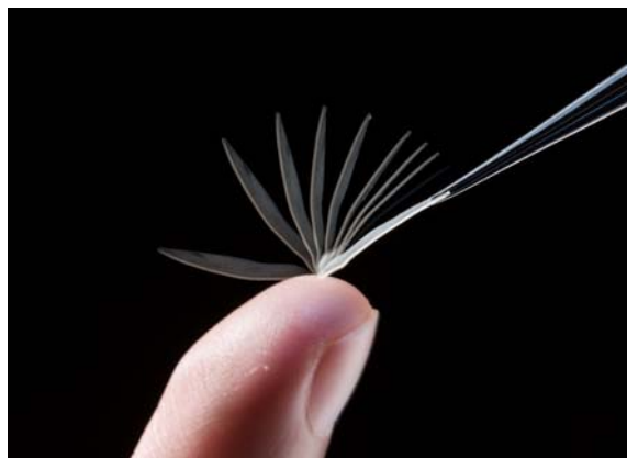
Figure 2. A shape-memory material can be deformed into a temporary shape that holds its form until it is triggered to revert to its permanent shape by application of heat, as shown in this multiple exposure photograph. The Anthamatten Group tuned such an elastomer to change its shape when heated to just beneath the human body temperature. Photo by J. Adam Fenster, University of Rochester
