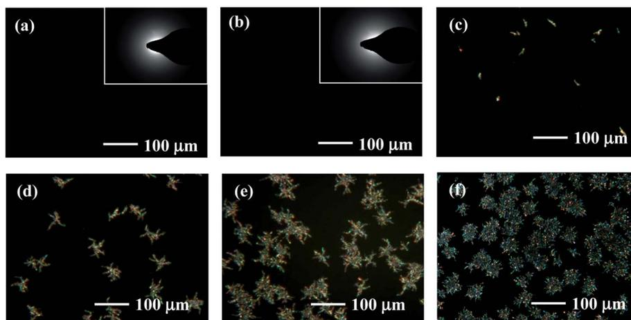
**Fig. 4** Polarizing optical micrographs of (a) TmPyPB annealed at 60 °C for up to 14 days, (b) ITO/MoO<sub>3</sub>/TAPC/**mCP-*g*-PhSiPh3:FIrpic**/TmPyPB annealed at 60 °C for up to 198 h, and ITO/MoO<sub>3</sub>/TAPC/**mCP:SiPh4:FIrpic**/TmPyPB annealed at 60 °C for (c) 1 h, (d) 2 h, (e) 3 h, and (f) 9 h. Insets in (a) and (b): electron diffraction images of TmPyPB and MoO<sub>3</sub>/TAPC/**mCP-*g*-PhSiPh3:FIrpic**/TmPyPB annealed at 60 °C for up to 14 days and 198 h, respectively.
