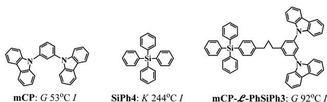
**Chart 1** Molecular structures of host materials with their thermal transition temperatures determined by DSC second heating scans. Symbols:  $G$ , glassy;  $K$ , crystalline; and  $I$ , isotropic.
